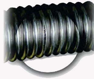
Circumferential cracks on the convolution are typically caused by high velocity flow rates
